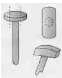
Grind pin head to shape
